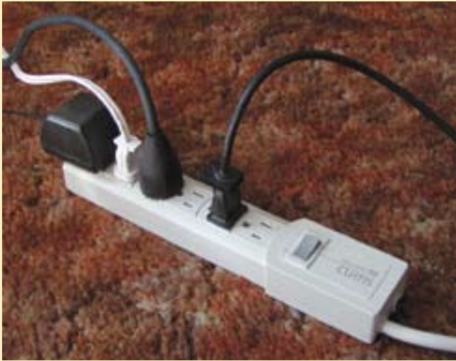
This plug strip is used to control multiple phantom loads with the flip of one switch.
